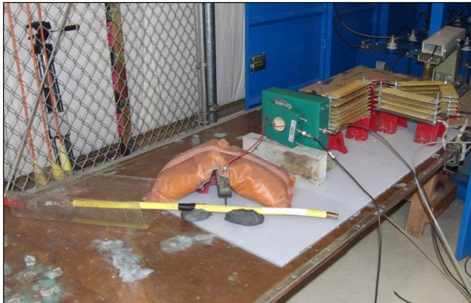
Figure 8 – Photograph of Typical Setup for LC1024 “Arcing Resistance” Tests, Non-Conductive Jacketed CSST Test Samples
