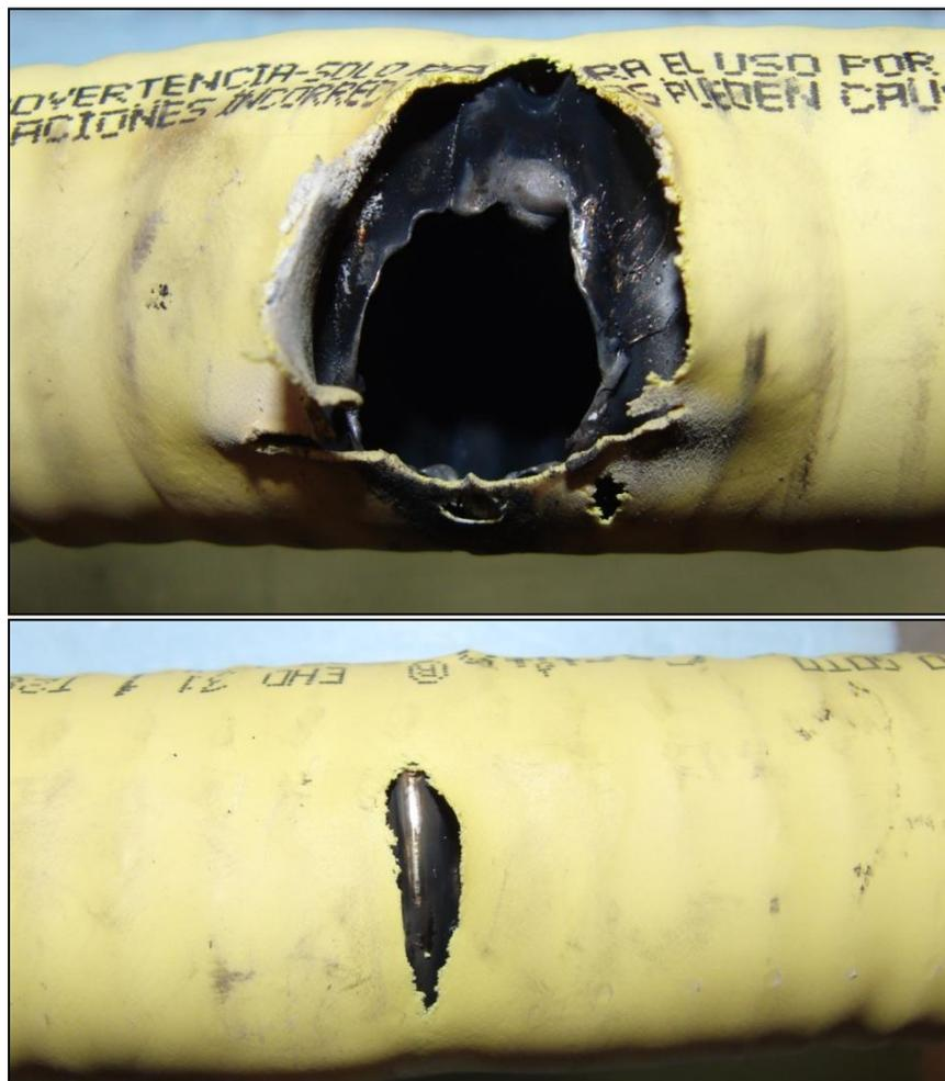
Figure 20 – Post-Test Photograph of Arc Discharge Area on 1.0” sized CSST, 41.2 Coulombs Total (Test No. 8)
