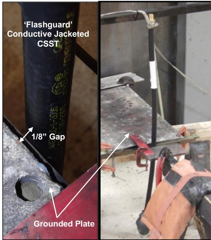
Figure 4 – Photograph of Typical Setup for LC1027 “Arcing Resistance, Direct Effects” Tests, Conductive Jacketed CSST Test Sample
