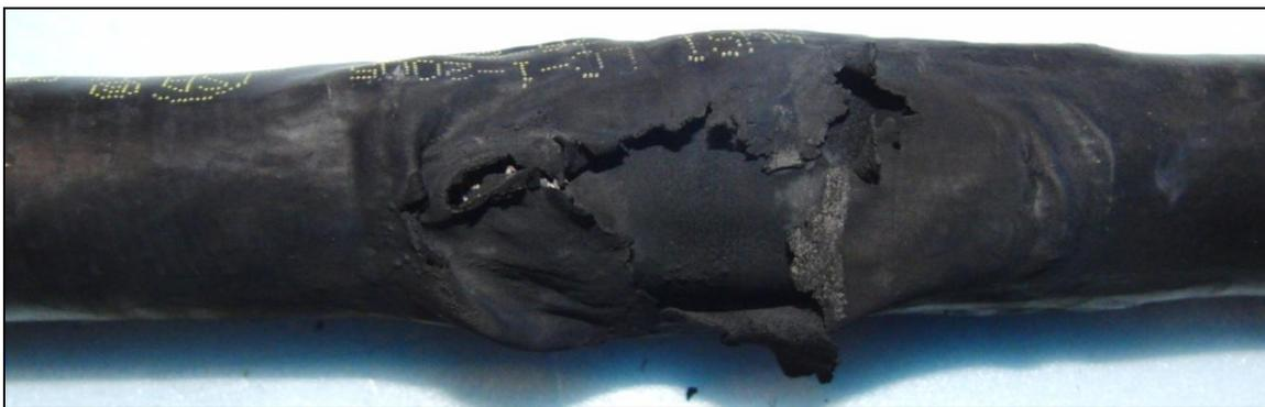
Figure 22 – Post-Test Photograph of Arc Discharge Area on 0.5” sized CSST, Conductive Jacket, 42.9 Coulombs Total (Test No. 7)
