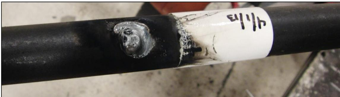
Figure 18 – Post-Test Photograph of Arc Discharge Area on Black Iron Pipe Section, 267.1 Coulombs Total (Test No. 5)
