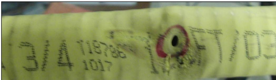
Figure 28 – Post-Test Photograph of Arc Discharge Area on 0.75” sized CSST, Non-Conductive Jacket w/ LP gas, 4.72 Coulombs Total (Test No. 18)
