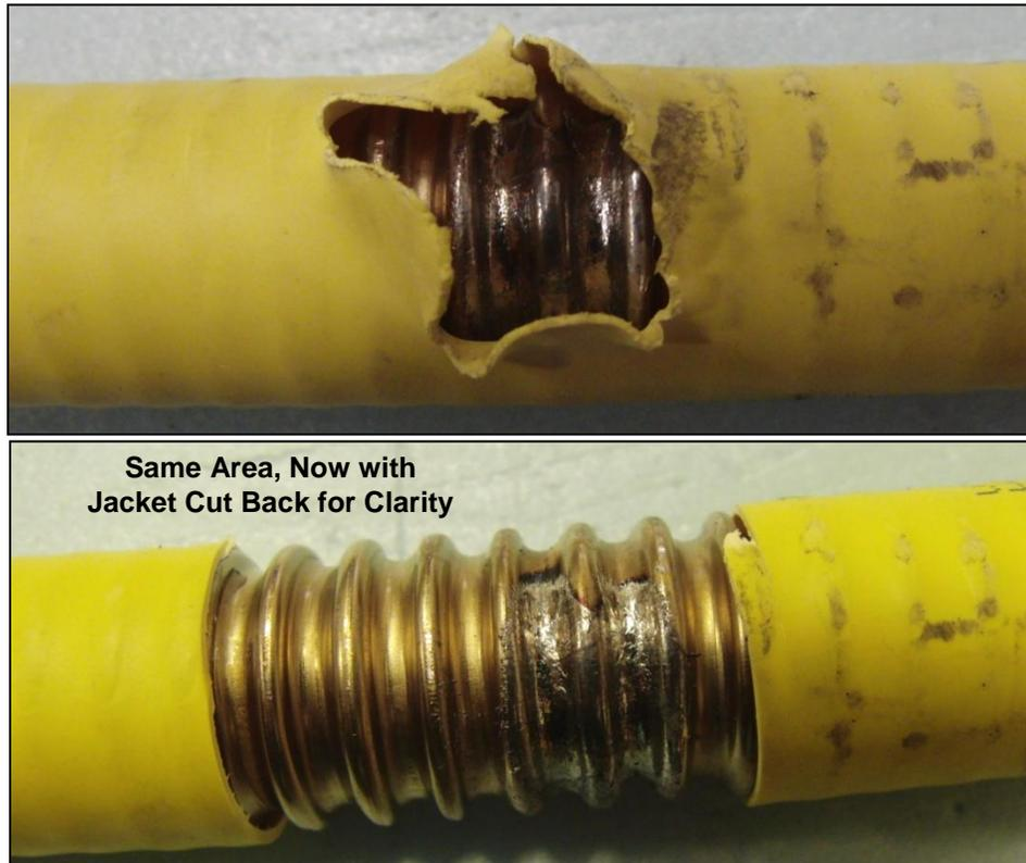
Figure 21 – Post-Test Photograph of Arc Discharge Area on 0.5” sized CSST, 2.86 Coulombs Total (Test No. 9)
