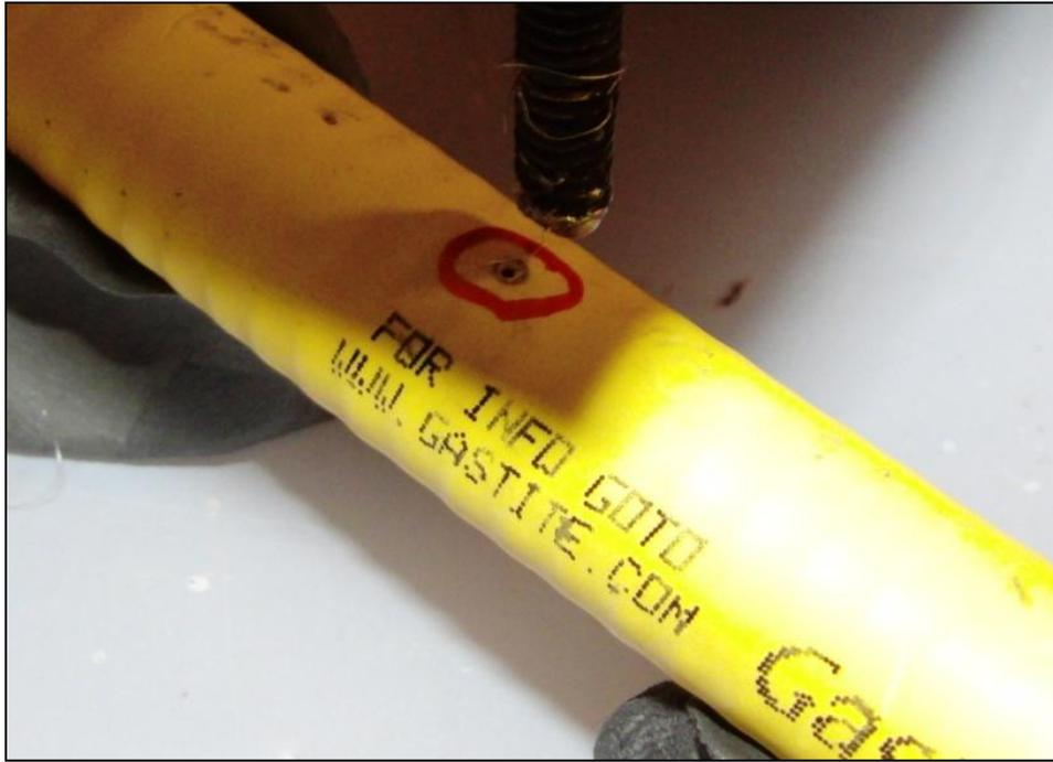
Figure 24 – Post-Test Photograph of Arc Discharge Area on 0.5" sized CSST, Non-Conductive Jacket, 1.96 Coulombs Total (Test No. 13)
