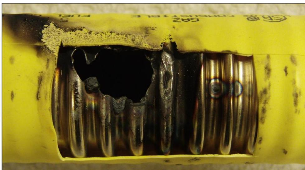
Figure 19 – Post-Test Photograph of Arc Discharge Area on 1.0" sized CSST, 38.8 Coulombs Total (Test No. 6)
