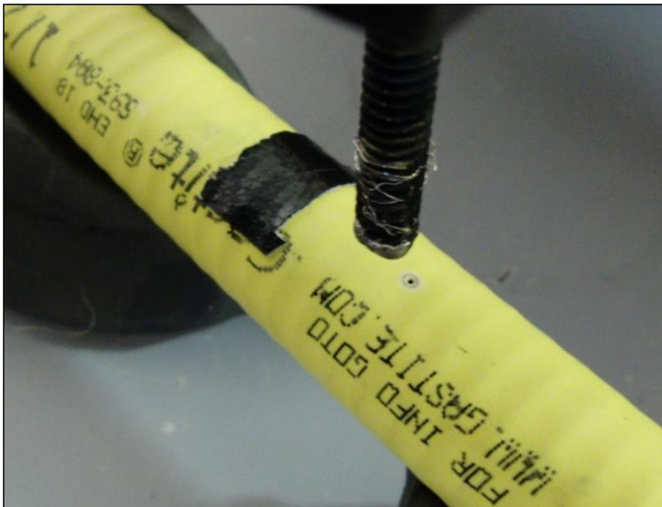
Figure 26 – Post-Test Photograph of Arc Discharge Area on 0.5” sized CSST, Non-Conductive Jacket, 0.76 Coulombs Total (Test No. 15)
