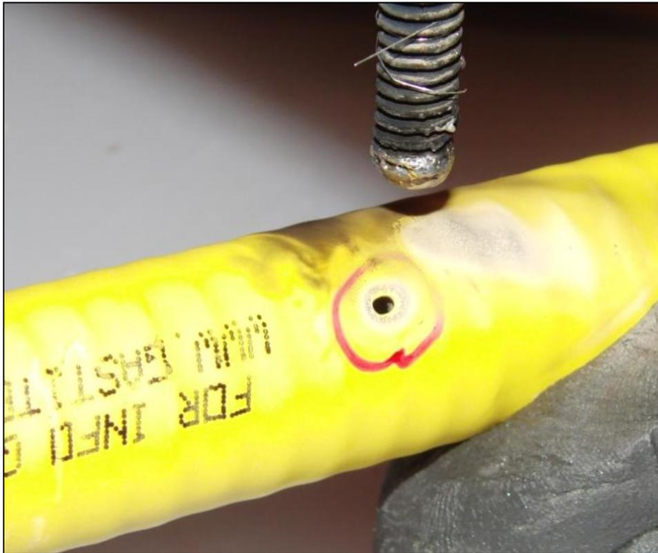
Figure 23 – Post-Test Photograph of Arc Discharge Area on 0.5" sized CSST, Non-Conductive Jacket, 3.62 Coulombs Total (Test No. 12)
