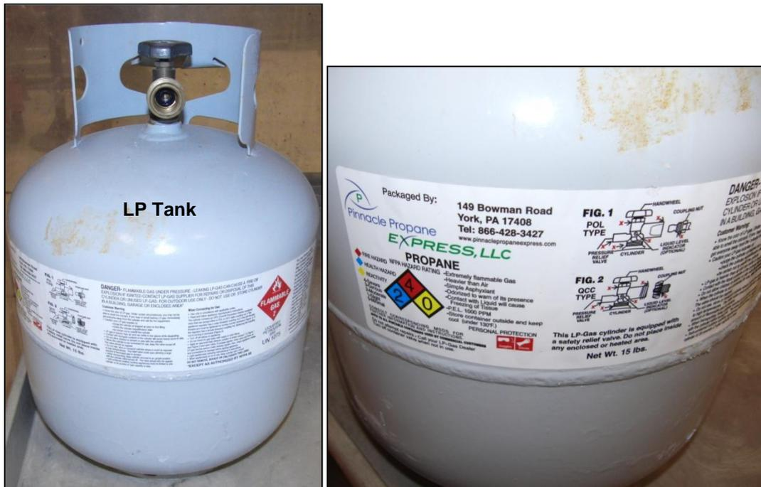
Figure 16 – Photograph of LP Tank Source for LC1024 “Arcing Resistance” Test using Pressurized Propane Gas
