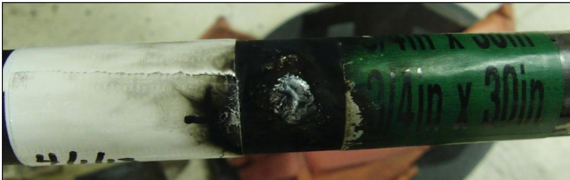
Figure 17 – Post-Test Photograph of Arc Discharge Area on Black Iron Pipe Section, 38.5 Coulombs Total (Test No. 4)
